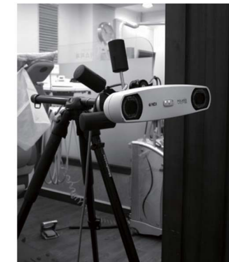
Fig 2. Optisches Tracking System (Polaris Vicra System, Northern Digital, Waterloo, Kanada)
